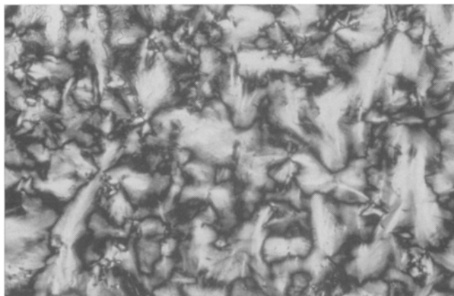
Fig. 5 Optical texture of pure monomeric DDAM at 75 °C observed under crossed polarising filters, magnification 480
